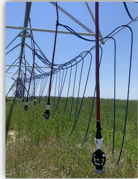
Figure 2. Precision mobile drip irrigation design by Netafim installed in a farmer's field in Southcentral Kansas.
